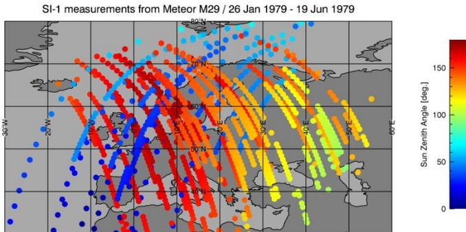
Figure 9: Sun zenith angle as computed for each spectra of the Meteor-29 dataset
