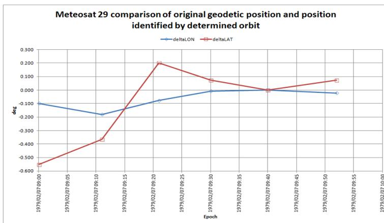
**Figure 8:** Difference in latitude (red line) and longitude (blue line) between simulated and actual positions of the measurements.
