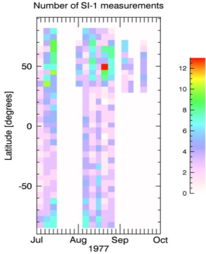
Figure 3: Latitude-time histogram of the number of SI-1 measurements performed from Meteor-28.
